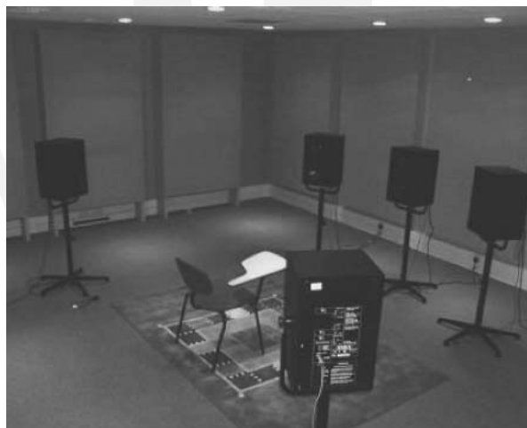
Fig. 5. Listening room finishes and five-channel loudspeaker arrangement.
