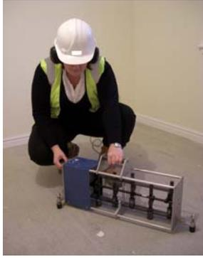
Fig. 4 Impact sound test being carried out
