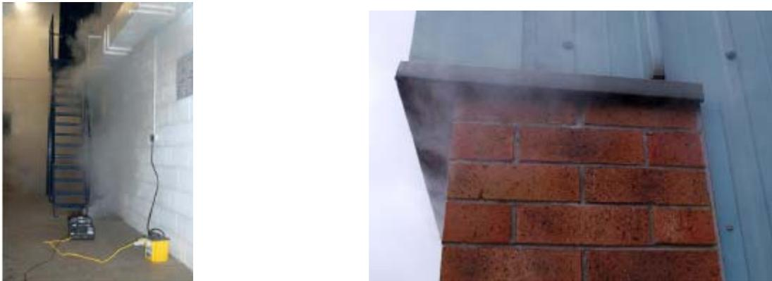
Fig. 8 Smoke testing
