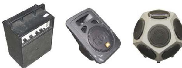
Fig. 3 Typical loudspeakers used during airborne sound insulation tests
